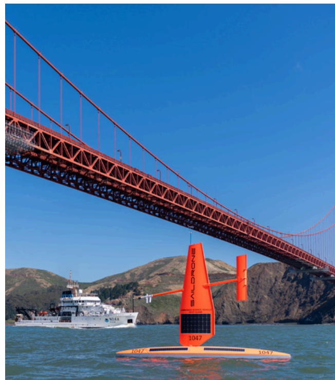
A Saildrone, an uncrewed surface vehicle, sails under the Golden Gate Bridge.
