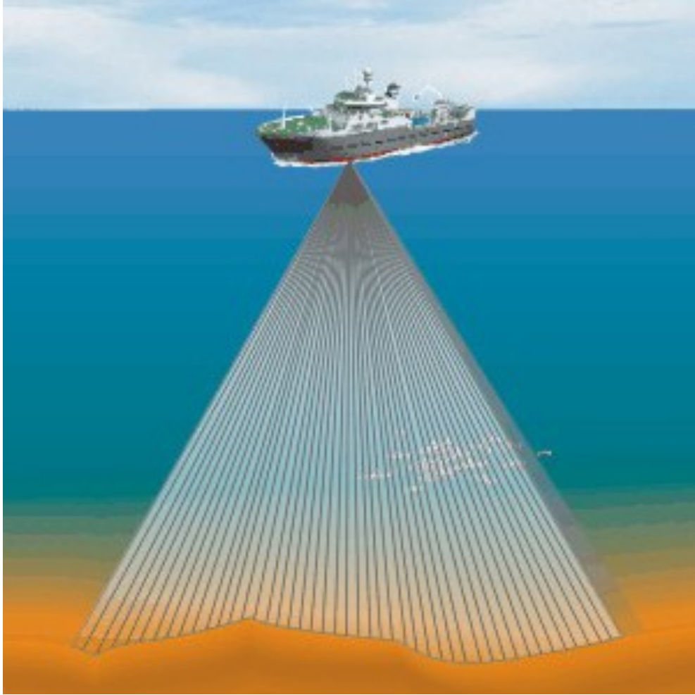
Figure A-18. Conceptual image of a multibeam echosounder
