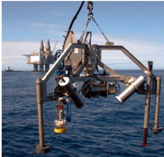
Figure A-20. A CamPod being deployed from a vessel
