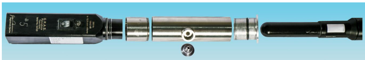
Figure 3. Split view of a G.R.A.S. 42AC pistonphone calibrator with an M36 hydrophone.
