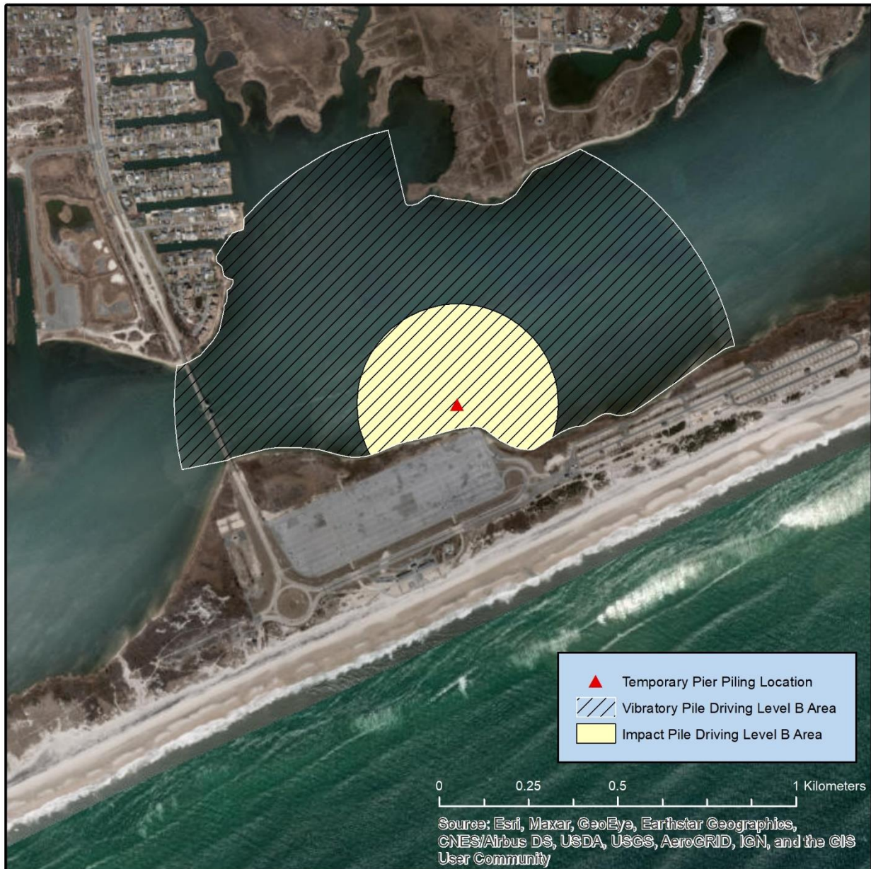
Figure 2. Location of the temporary pier and areas of water potential exposed above Level B thresholds from vibratory and impact pile driving.
