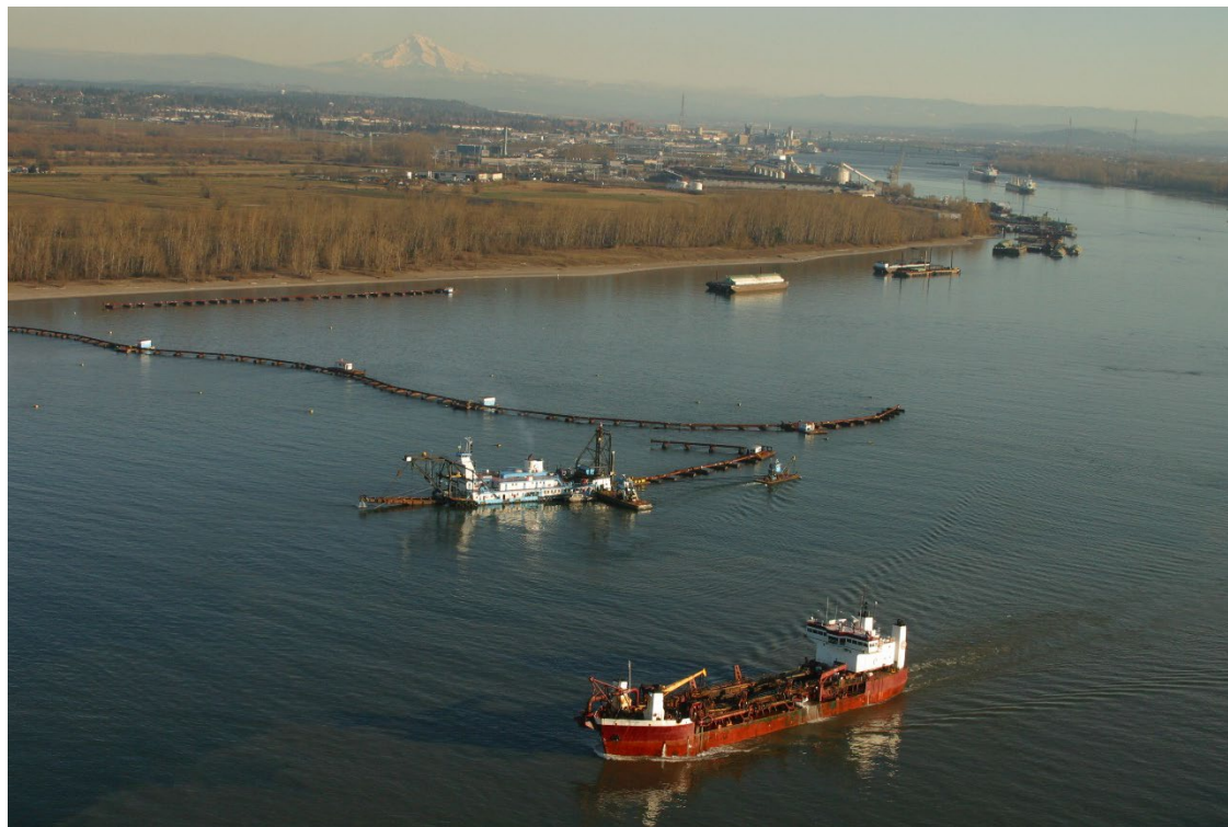
Figure 1-5. Photograph of actual pipeline (center) and hopper (bottom) dredges.
