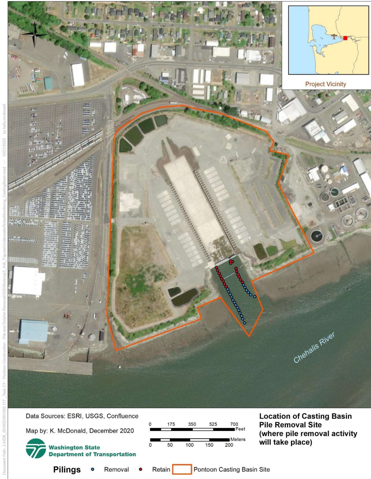
Figure 2. Location of 19 Pilings that were Removed
