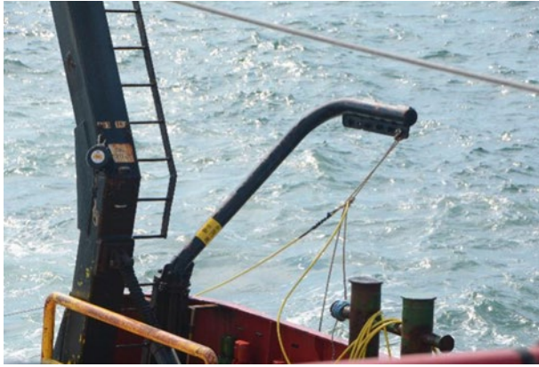
Figure 3: Chinese finger attached to hydrophone cable tow point leading out
