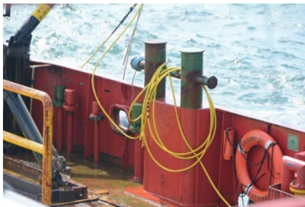
Figure 2: Hydrophone cable deployed, and tow cable stowed on the bollard
