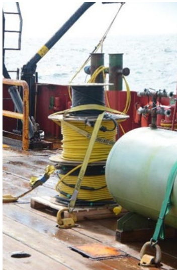
Figure 4: Deck cable, main and spare hydrophone cable and two cable secured
