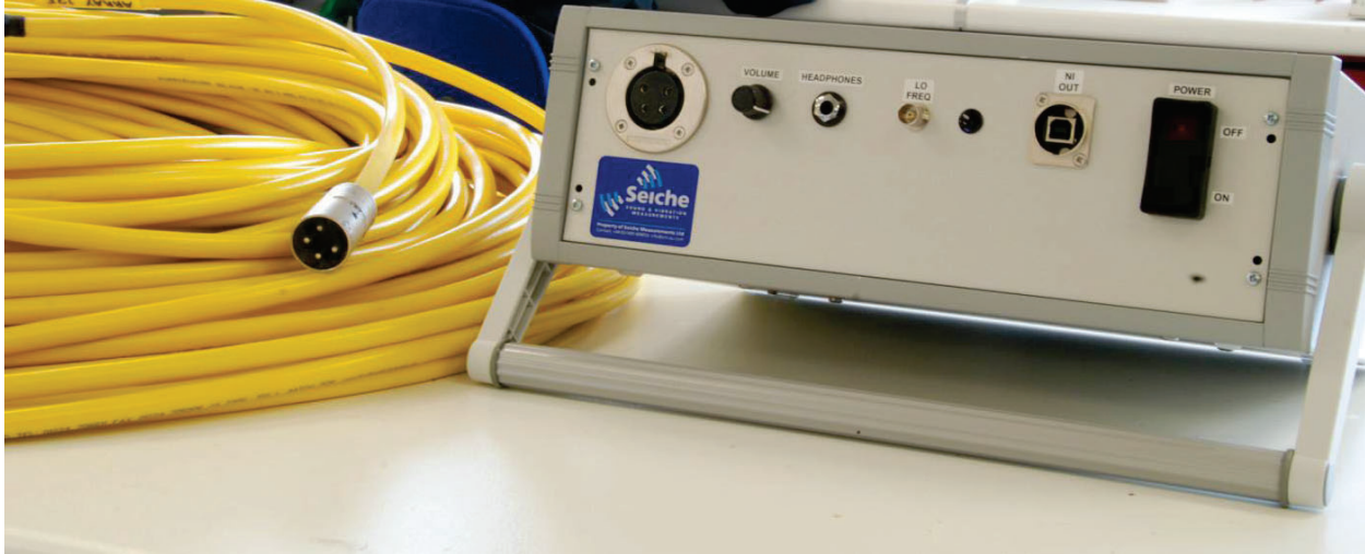
Figure 1: Electrical processing Unit and hydrophone array cable
