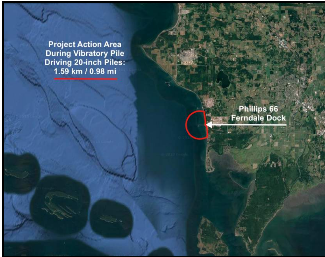
Figure 1. Project action area when driving 20-inch steel piles, generating underwater noise greater than 120 dB SPL.
