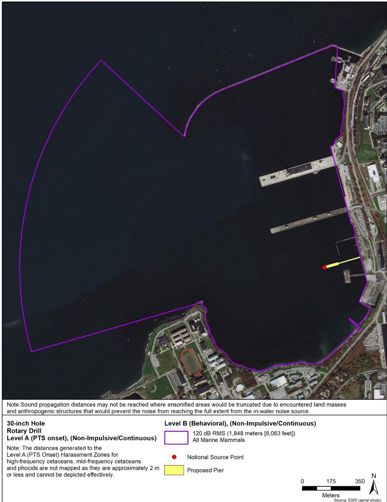
Figure 6-20 Level B (Behavioral) Harassment Zone from Rotary Drilling at the Pier – Hole for 30-inch Steel Pipe
