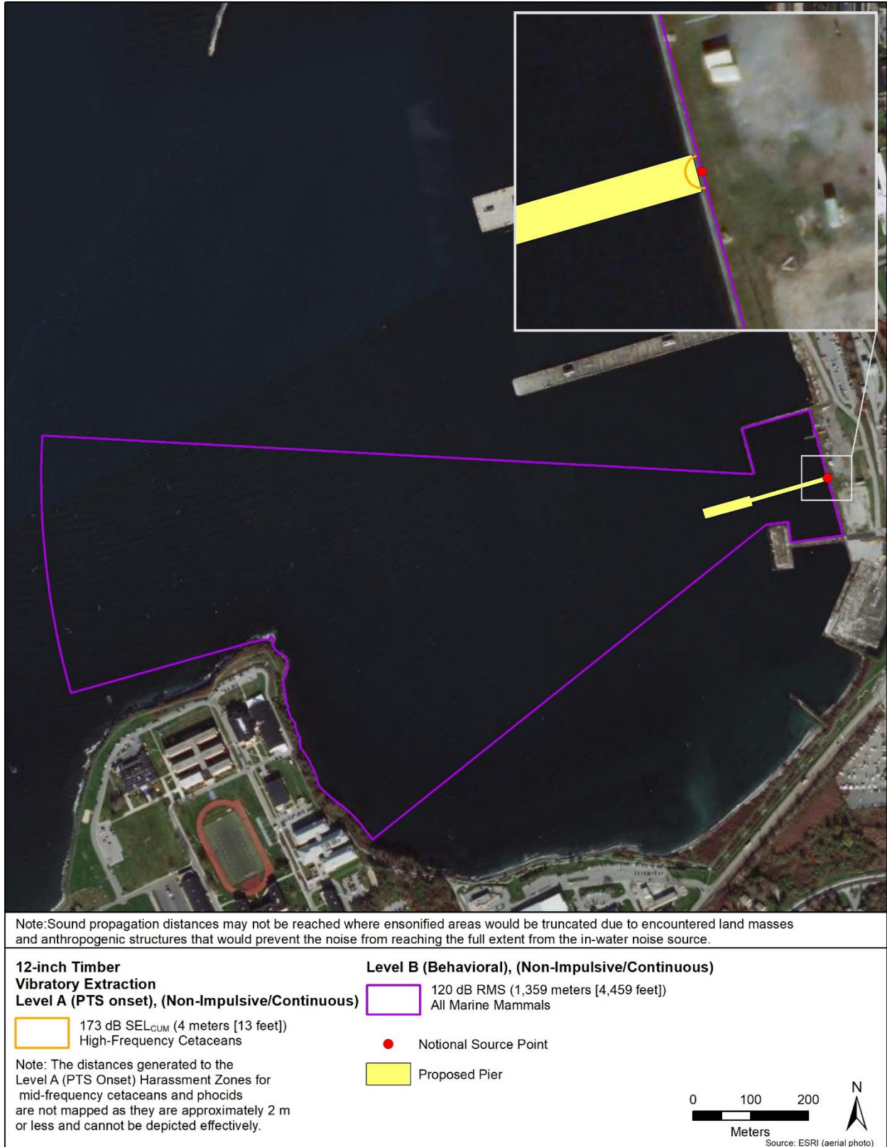
Figure 6-10 Level A (PTS Onset) and Level B (Behavioral) Harassment Zones from Vibratory Extraction Activity for Floating Dock Demolition – 12-inch Timber Guide Piles
