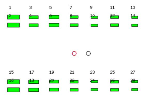
The array described above consists of 28 air guns and has a total volume of 5,200 cubic inches. There will be two source vessels. Each source vessel will tow three of the 5,200 cu. in. arrays at a crossline distance of 100m. Hence, the distance between the outer arrays is 200m. The shot interval for each source is 50m which means that a source will fire every 16.6666m.
