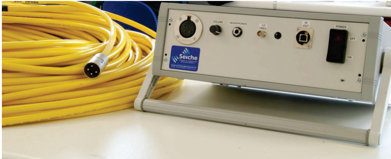
Figure 1: Electrical processing Unit and hydrophone array cable
