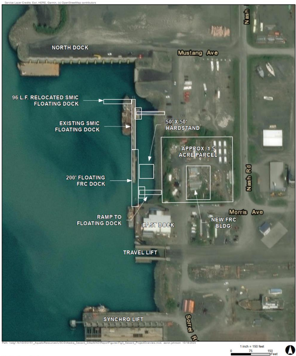
Figure 1-3 Seward Proposed Project Components
