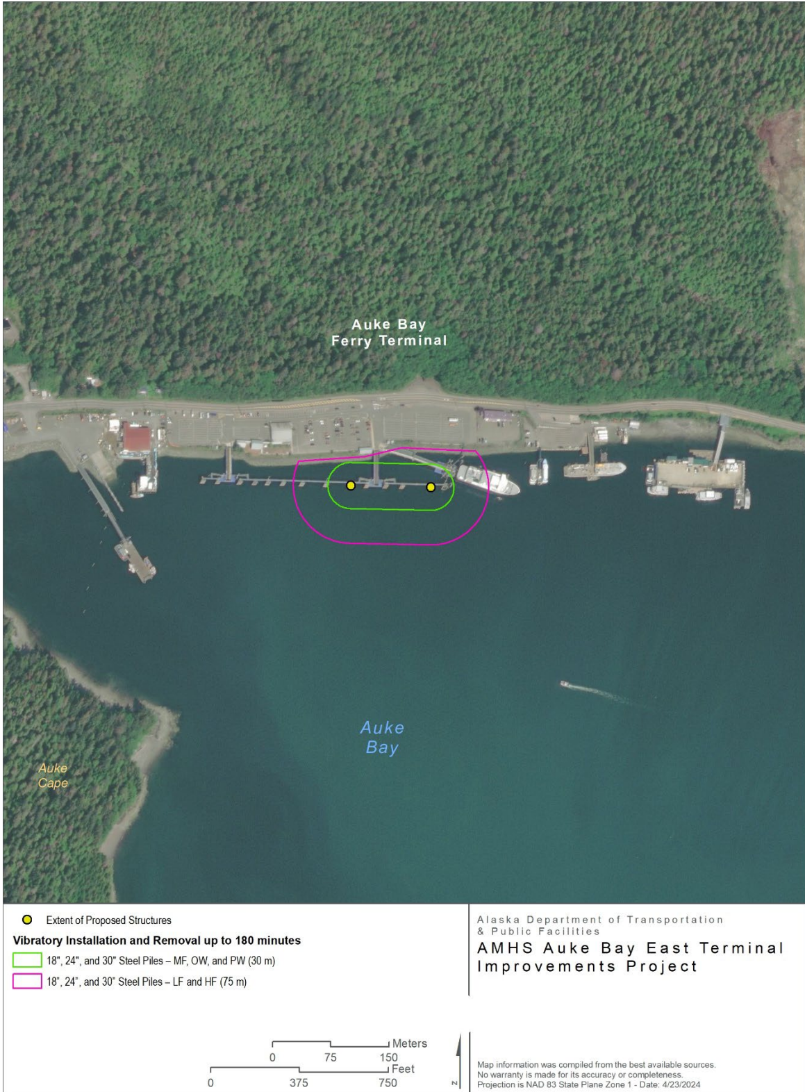
Figure 2-1. Shutdown Zones during Vibratory Pile Installation and Removal at Auke Bay East Ferry Terminal
