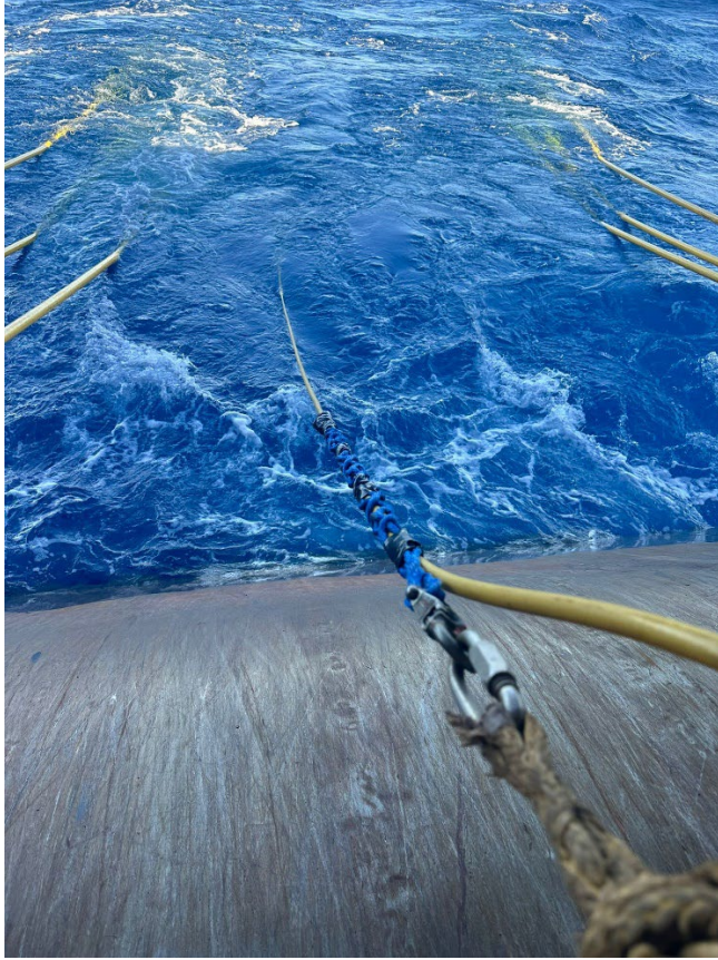
Figure 6. Chinese finger at 80-meter mark attached to gate
