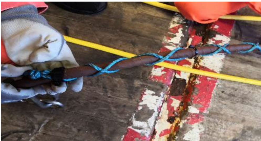
Figure 4: A Chinese finger was attached to the 70-meter mark as a tow point creating a more even spread of the tension.
