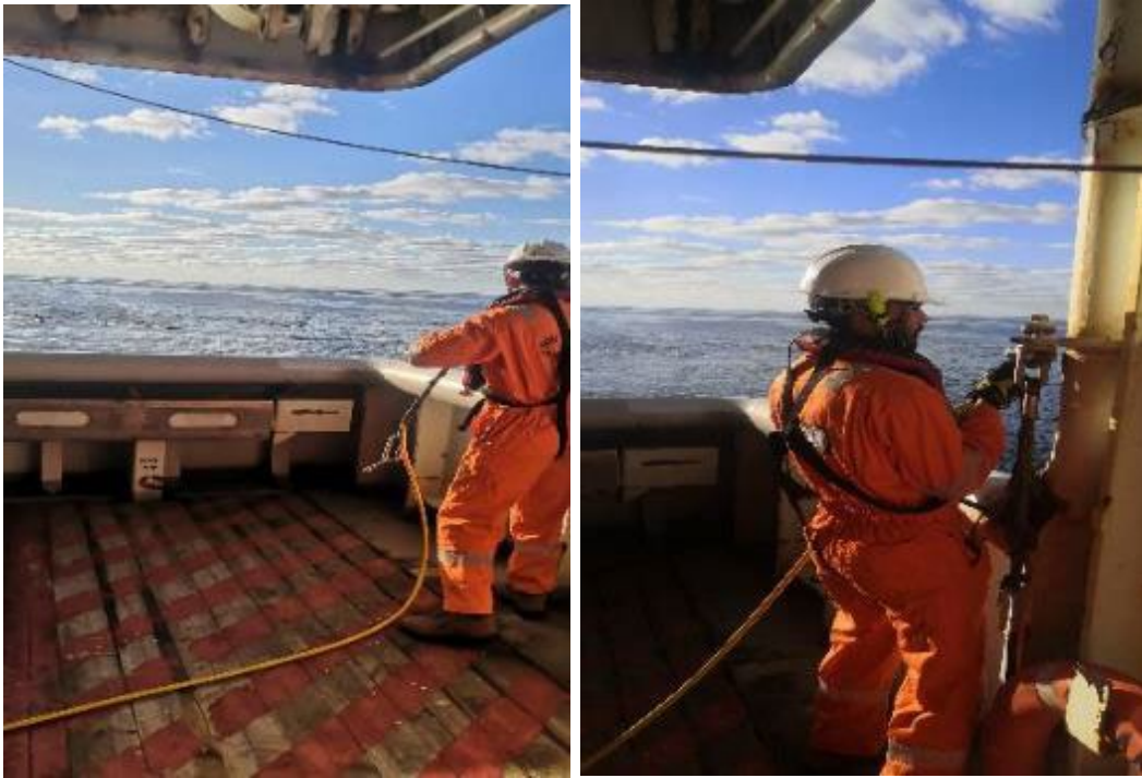
Figure 3: Hydrophone cable deployed from streamer deck portside lead-in (3A) and portside anchor point (3B).
