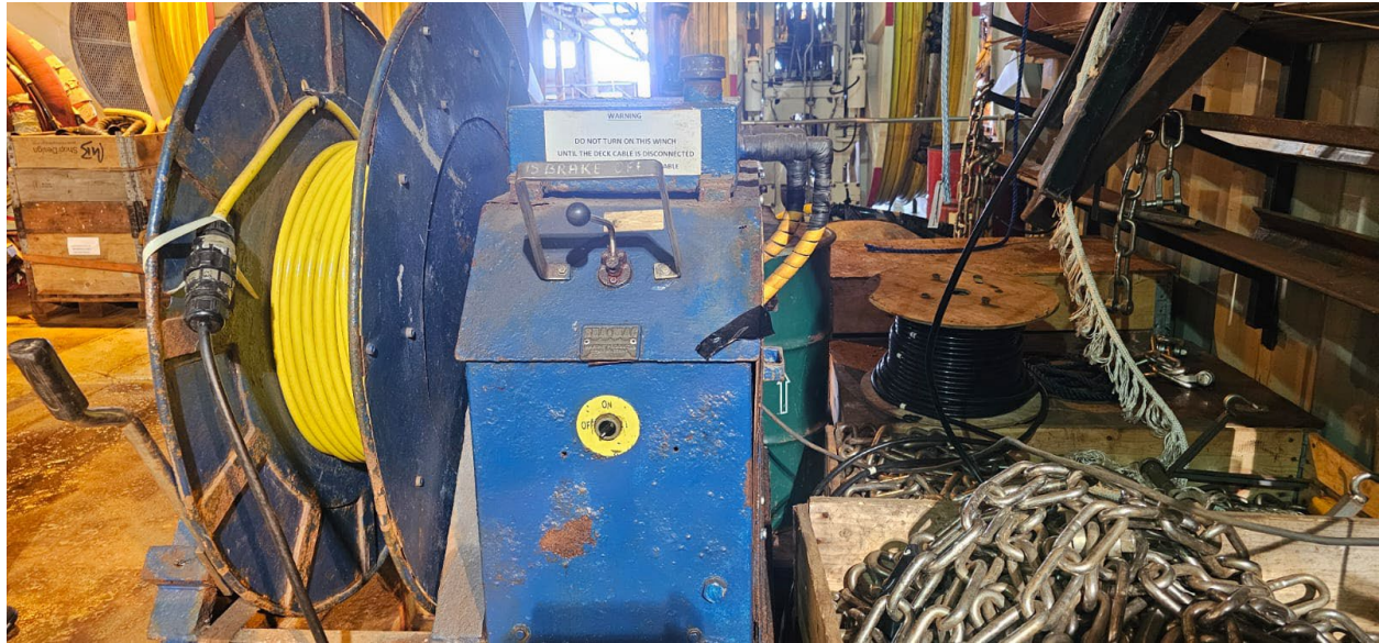
Figure 2. Tow cable mounted on winch and connected to the deck cable (bottom right side).
