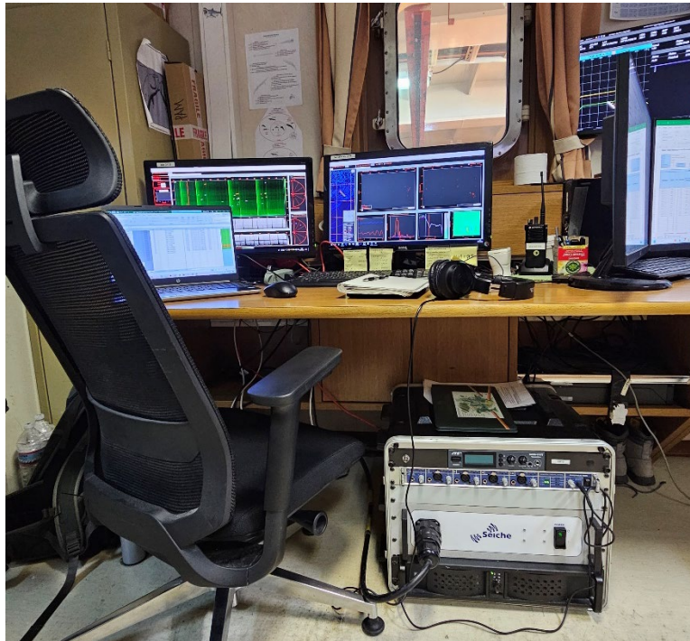
Figure 7: Passive acoustic monitoring station in instrument room.
