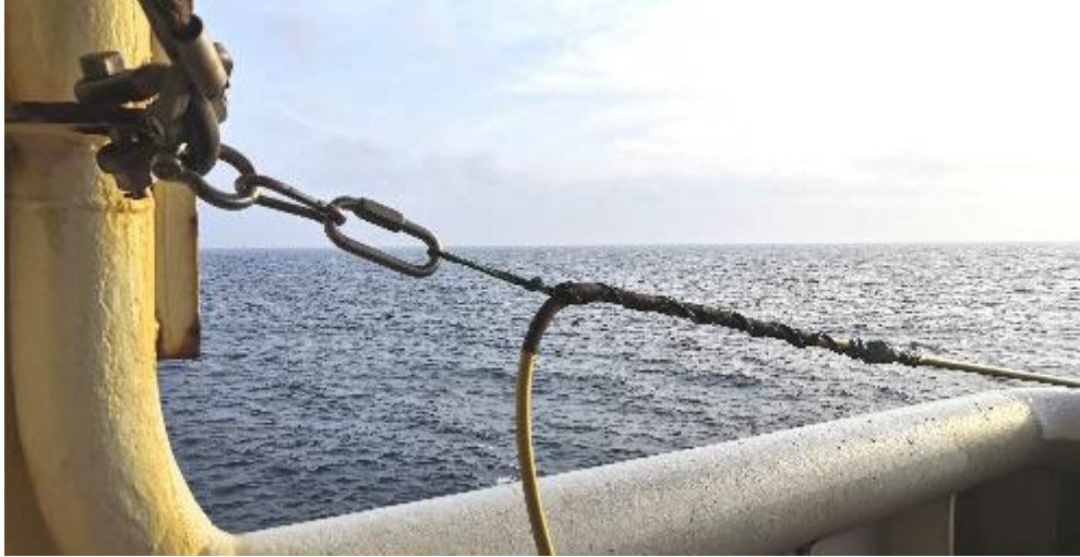
Figure 5: Chinese finger attached to the anchor point on the starboard side on the R/V Oceanic Champion.
