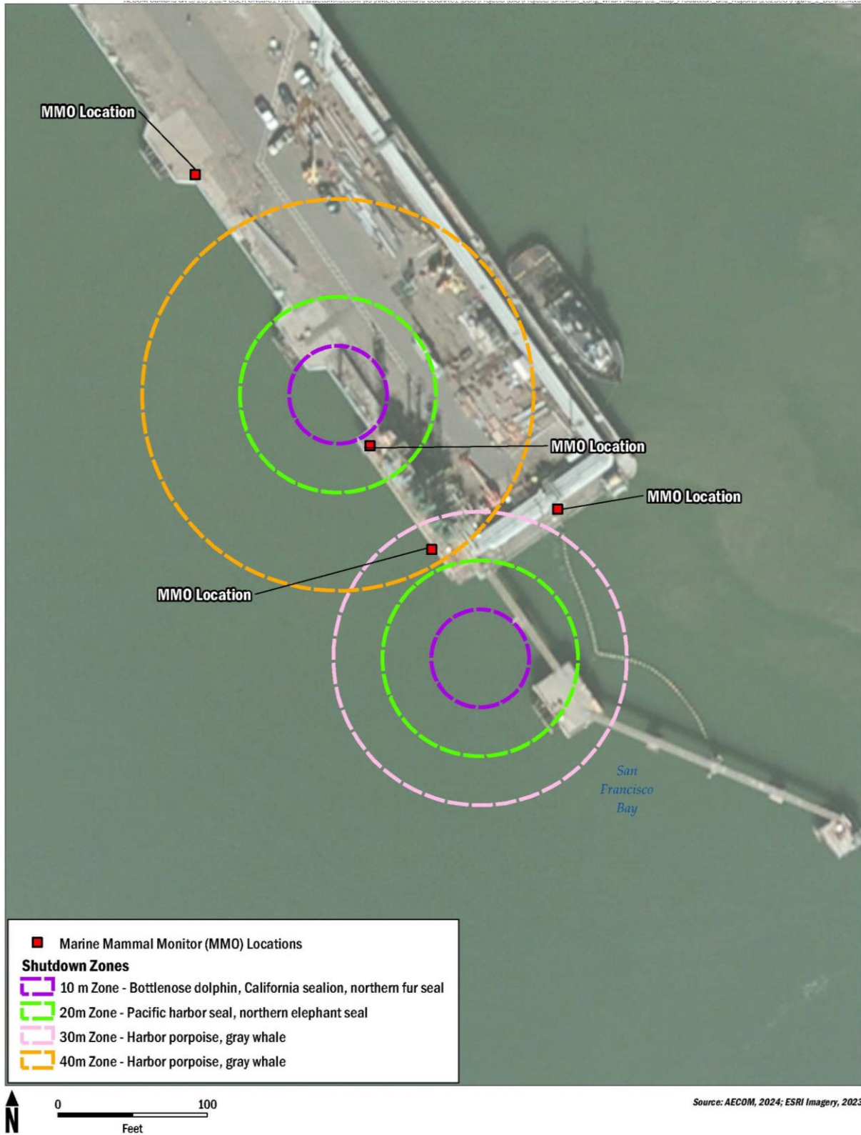
Figure 2 Berth 1 Shutdown Zones for 24-inch Concrete Pile Installation (top) and 36-inch Steel Pile Installation and Extraction (bottom)
