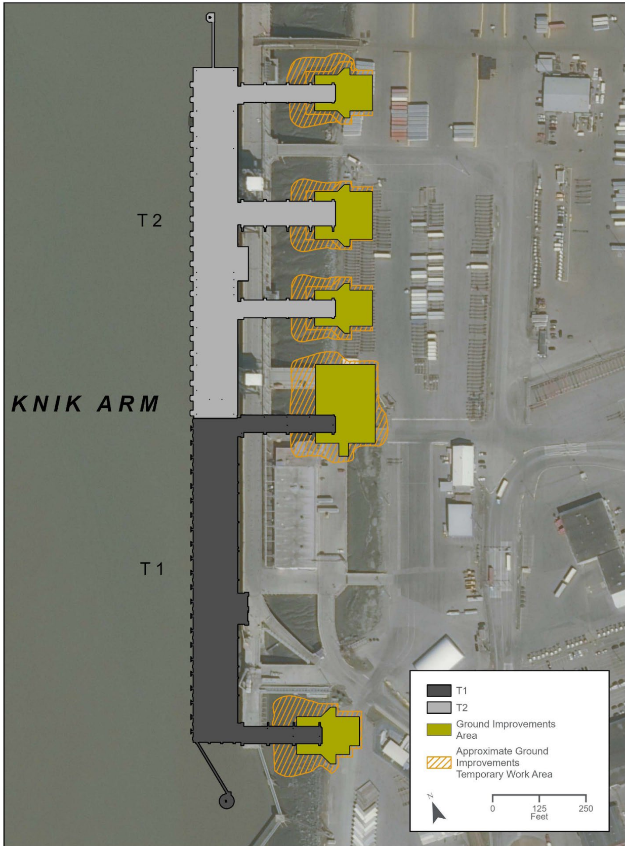
Figure 1-2. Component 1: Ground Improvement Locations and Approximate Areas
