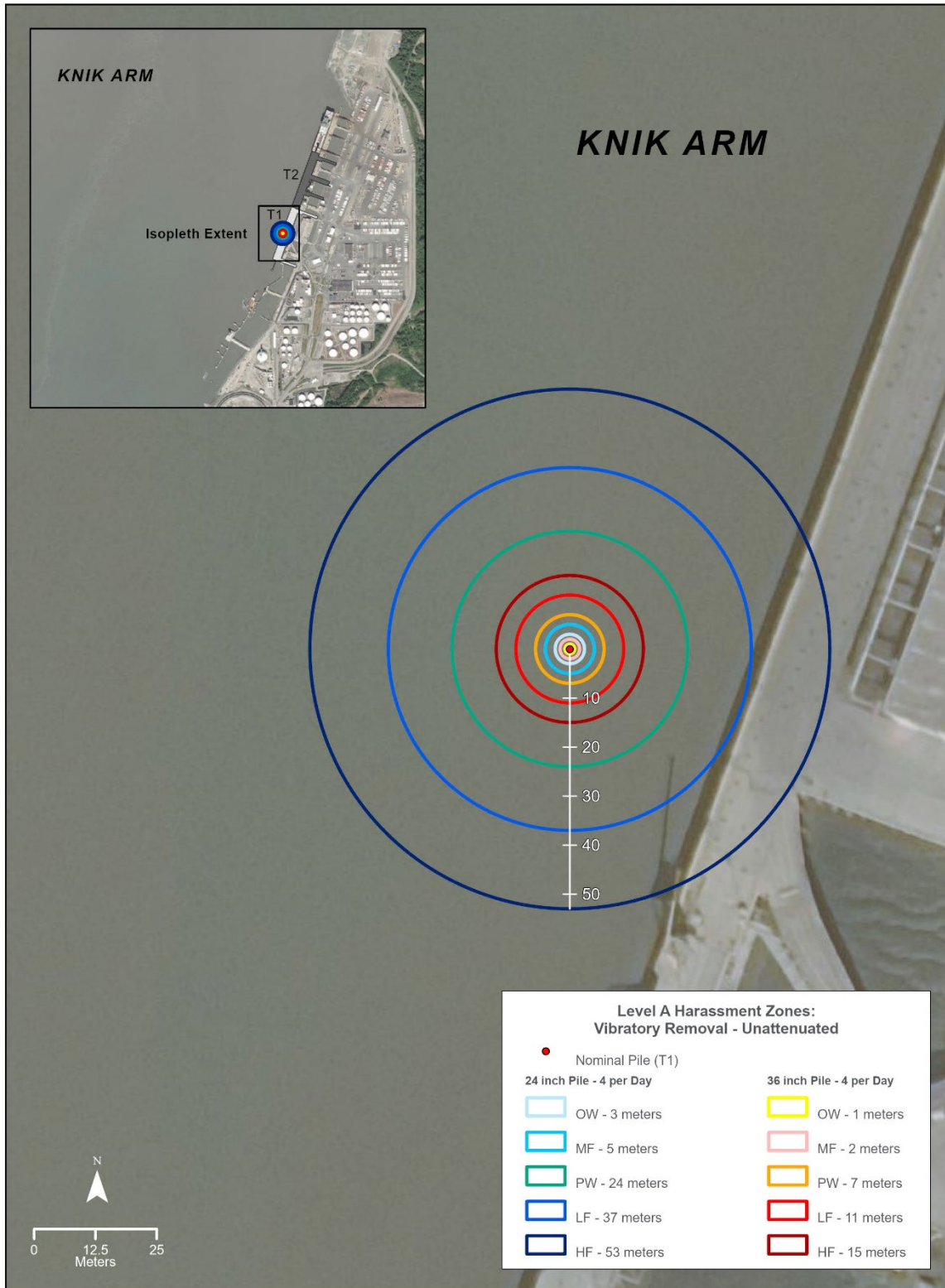
Figure 6-8. Level A Harassment Isopleths for Vibratory Pile Removal (Unattenuated)
