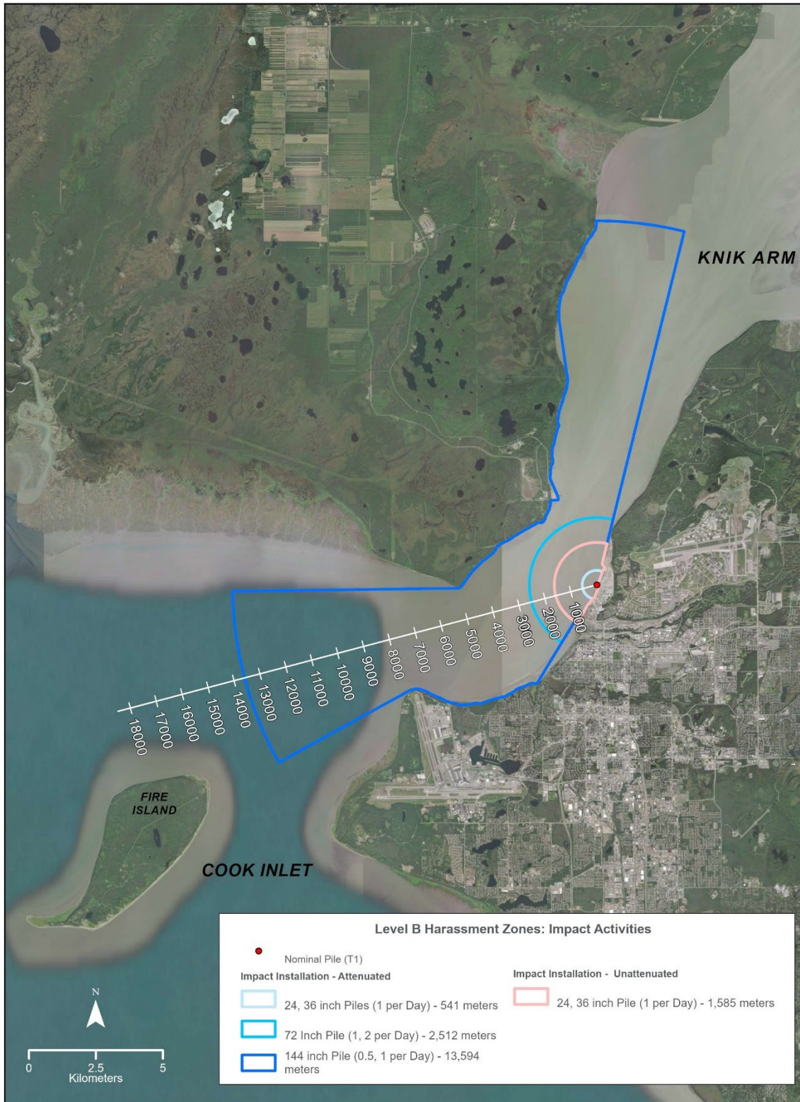
Figure 6-9. Level B Harassment Isopleths for All Pile Sizes for Impact Installation (Attenuated and Unattenuated)
