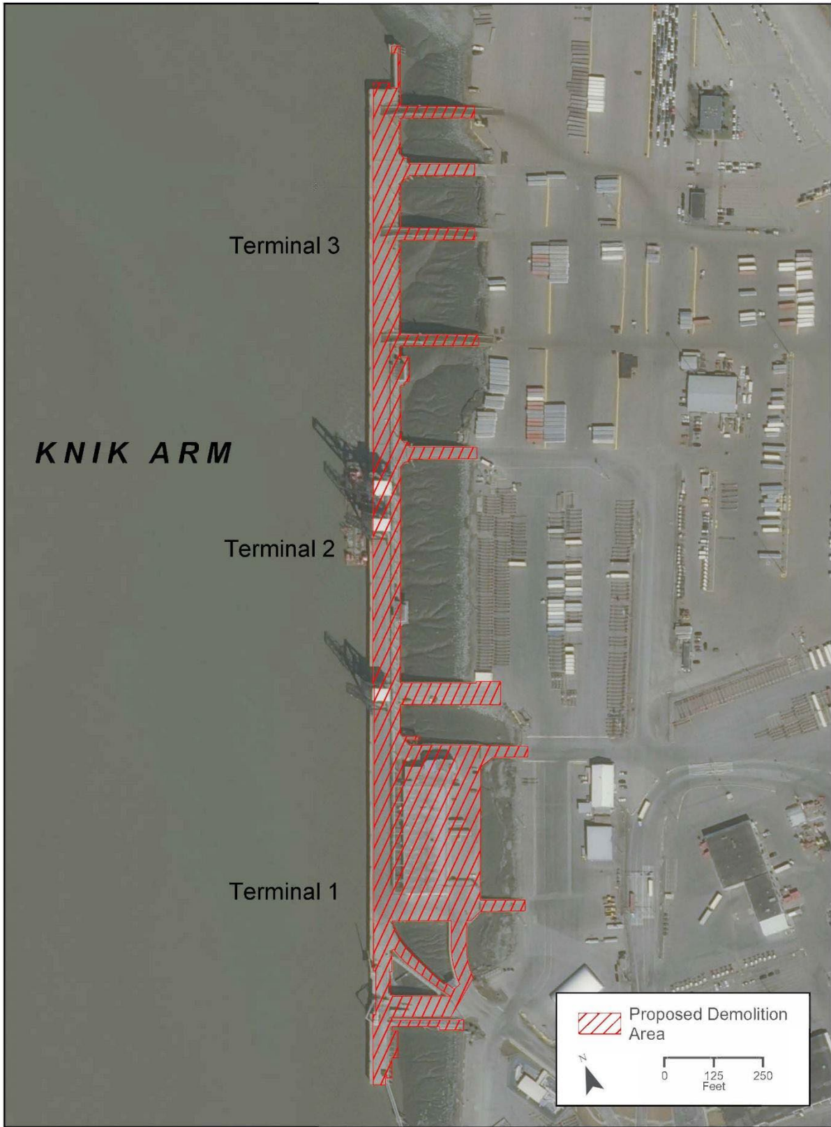
Figure 2-5. Component 4: Demolition of Existing Terminals
