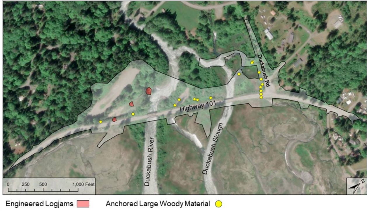
Figure 9. Installation locations of engineered logjams and anchored large woody material
