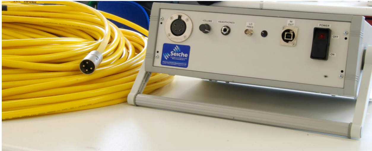
Figure 1: Electrical processing Unit and hydrophone array cable
