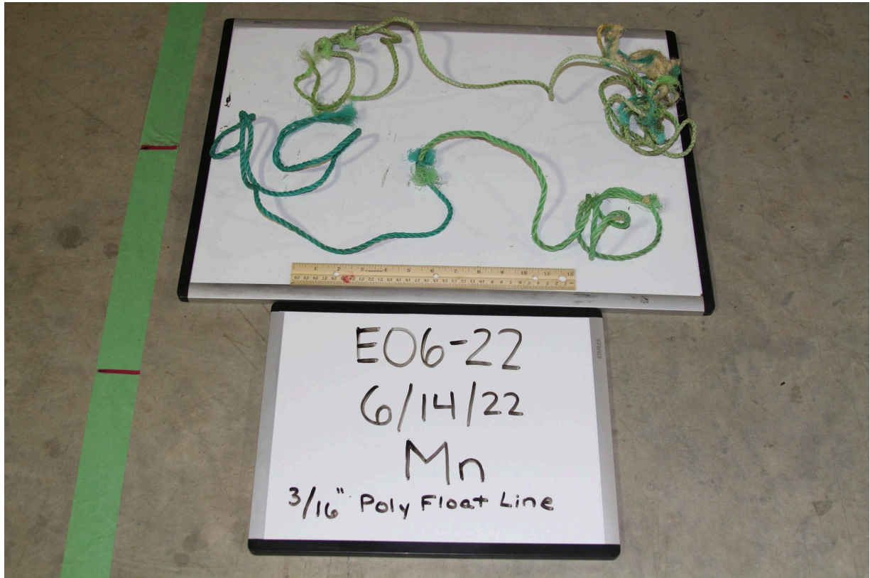
Photo 5: Small portion of recovered 3/16" rope.
