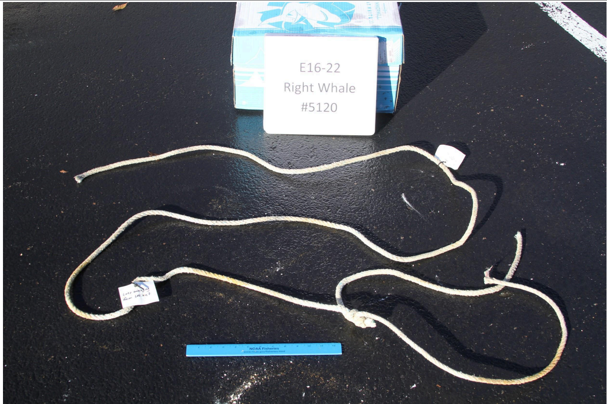
Photo 7: Portion of gear recovered on 2/02/24 from IFAW; two different types of rope with carrick bend. Photo from NOAA Fisheries.
