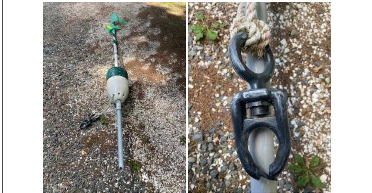
Photo 1: High flyer buoy with 600# broken weak link.
